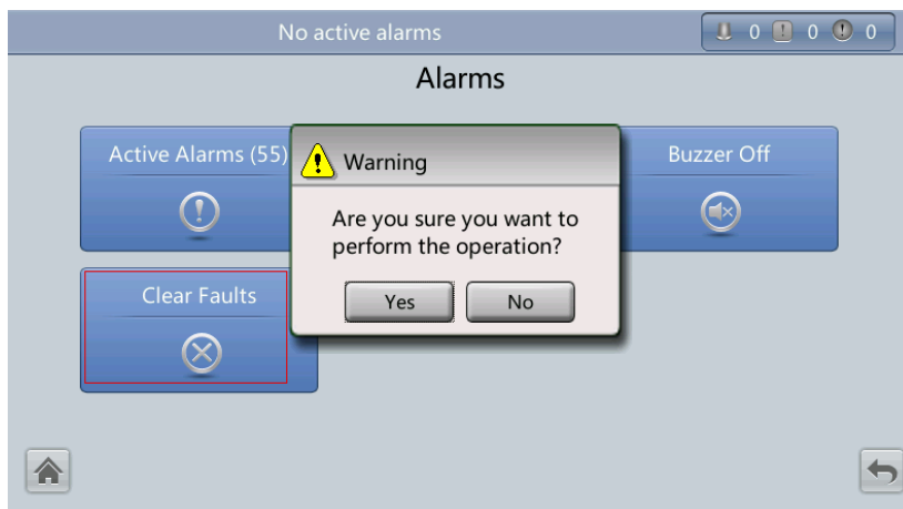
Figure 4-21 Clear Faults screen
