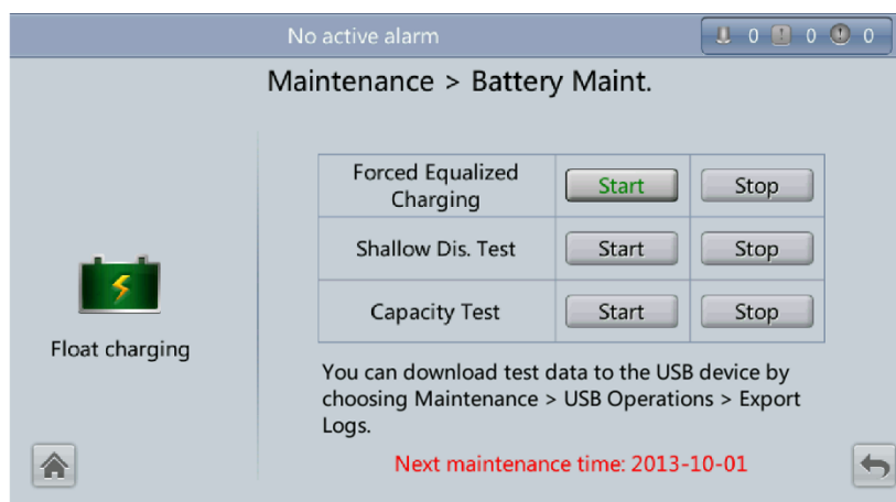
Figure 4-54 Battery Maint. screen
